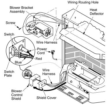
Figure 16 - Installing Blower Bracket Assembly
